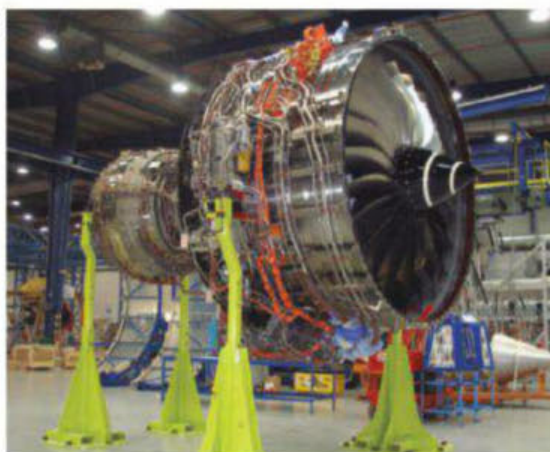
The first flight-compliant Rolls-Royce Trent XWB-84 for the A350-900 is prepared for aircraft installation in Toulouse.
