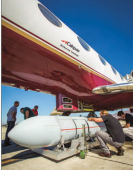
Raytheon's Next Generation Jammer pod for U.S. Navy uses AESAs with gallium-nitride power electronics.
