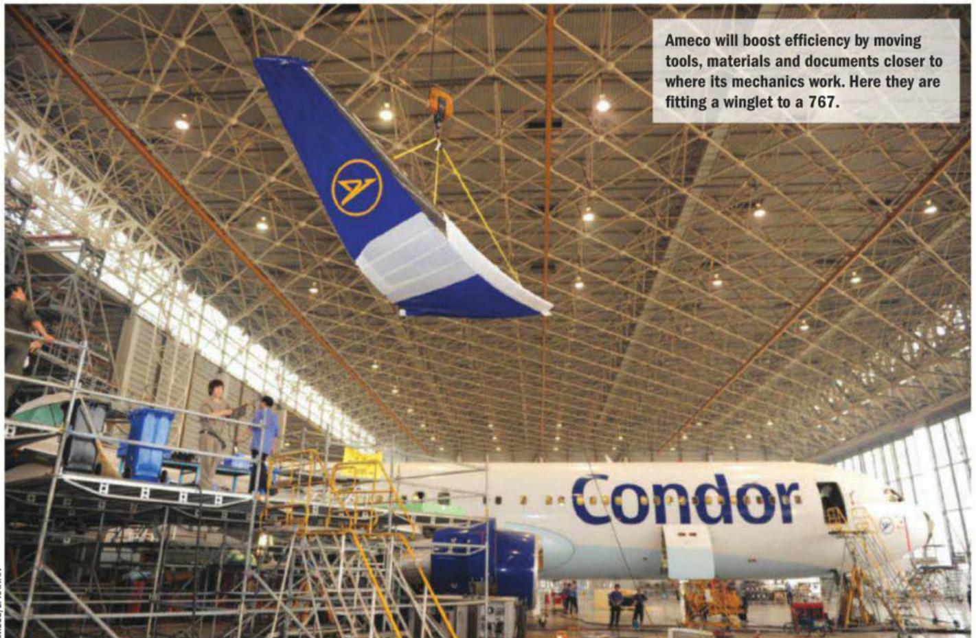
Ameco will boost efficiency by moving tools, materials and documents closer to where its mechanics work. Here they are fitting a winglet to a 767.
