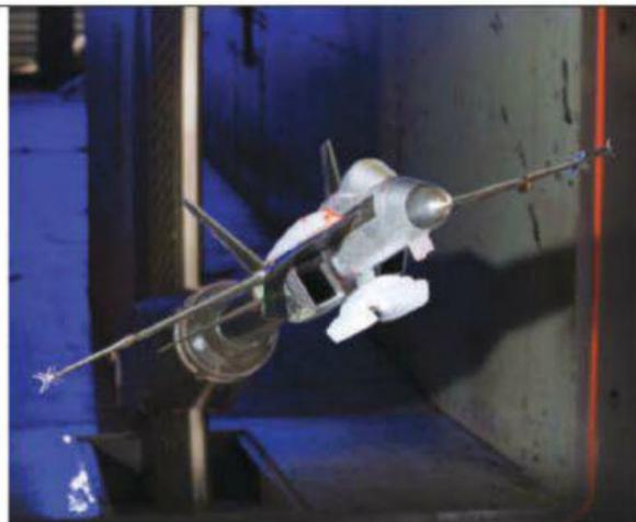
**A Super Hornet wind tunnel model displays an exterior weapons bay that reduces F/A-18E/F radar reflectivity.**
