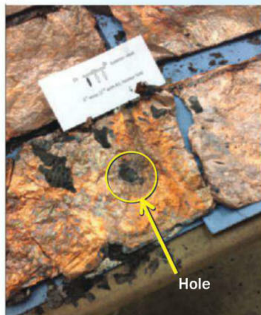
This hole in an electrode from the failed Japan Airlines battery indicates an internal short circuit.
