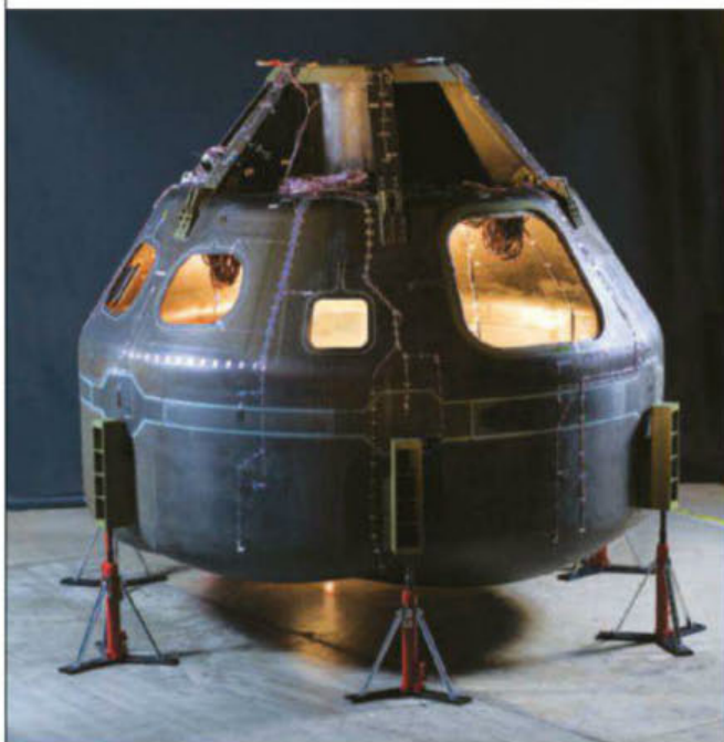
The ATK/Astrium Liberty launch system would carry crews in a composite version of the aluminum pressure vessel built for NASA’s Orion.
