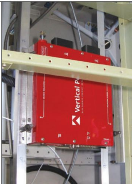
Vertical Power’s VP-X electronic circuit-breaker system, mounted below the floor boards, creates a smart power distribution system for experimental and light sport aircraft.
