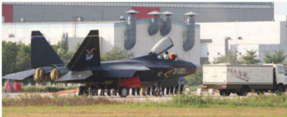
The tall vertical tails and clipped-delta wings of the J-31 recall the Lockheed Martin F-22, but the Chinese aircraft is smaller and lighter.
