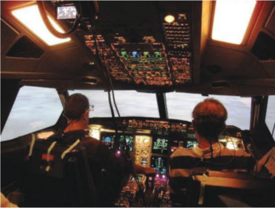
French investigators used flight simulators with eye and head-tracking devices to analyze how Boeing 777 and Airbus A330 pilots react to go-around scenarios.
