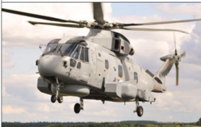
The AESA radars fit inside the two pods, pictured here in an early prototype configuration on a Royal Navy Merlin Mk. 2 ASW helicopter.
