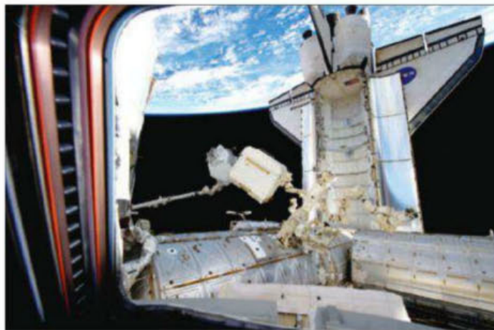
Dextre grasps a white cargo transport container from its perch atop the Destiny laboratory module as Canadarm2 pulls the Alpha Magnetic Spectrometer from Endeavour's cargo bay during the STS-124 mission.
