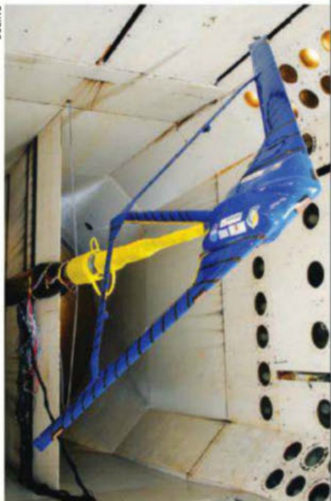
A Boeing joined-wing, SensorCraft, undergoes testing at NASA Langley's 16 X 16-ft. wind tunnel in 2010.
