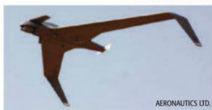
Orbiter 3 from Aeronautics Ltd. uses the 5-kg TD-Stamp payload with gyro-stabilized imaging.
