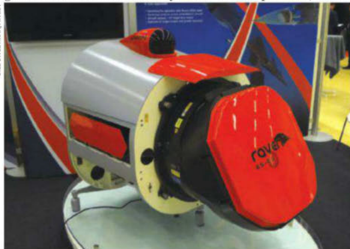
Mockup of Selex Galileo sensor package for JAS 39E/F shows single-rotation repositioner and side-looking phased-array IFF antennas.
