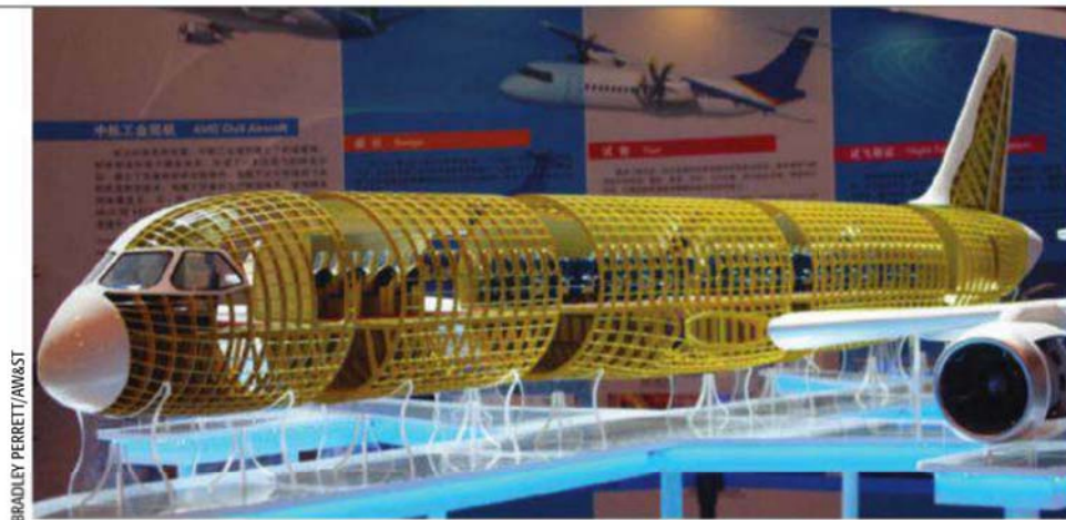
Although Avic has exhibited this structural scheme for the C919, wing and fuselage materials have not been decided.
