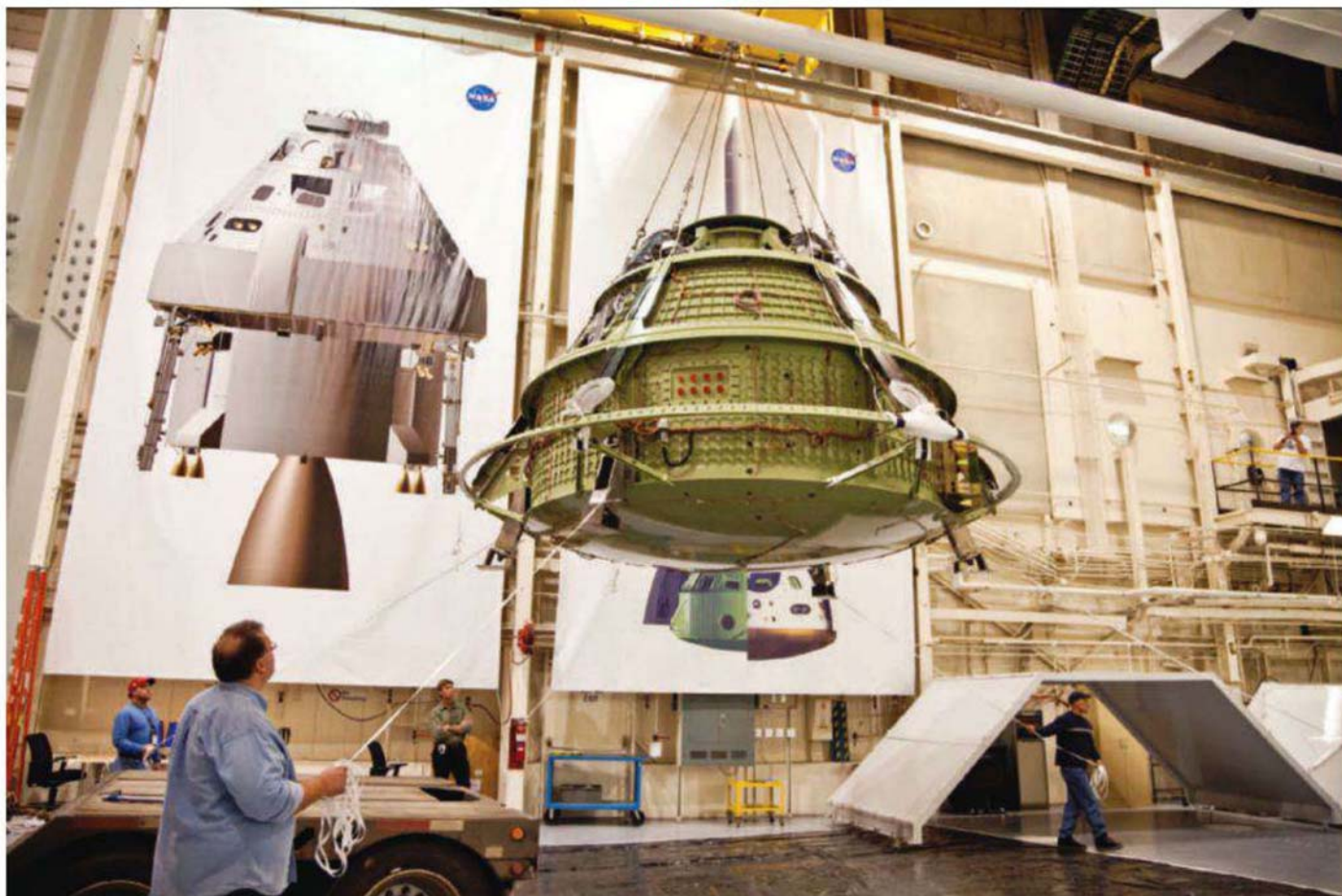
The first Orion test article arrives at Lockheed Martin's Denver facility, where it is being fitted with its thermal protection system prior to ground testing.
