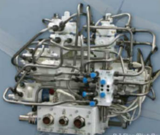
B-1 Flap/Slat Power Drive Unit
