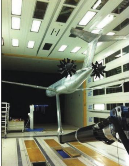
Wind-tunnel tests indicate aircraft powered by open-rotor engines will meet noise limits.
