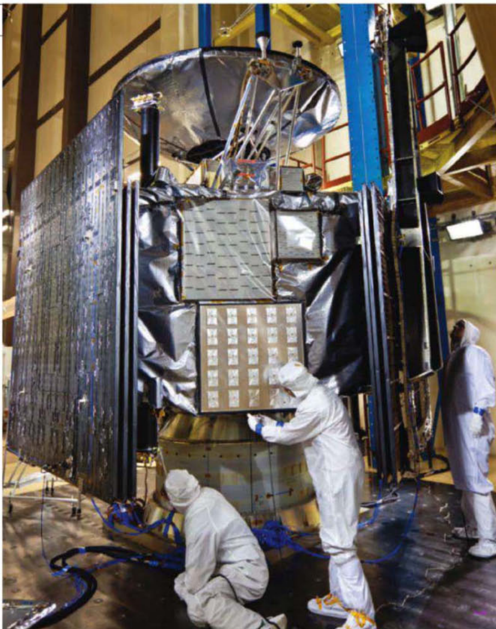
Flight-ready Juno spacecraft underwent acoustic testing at Lockheed Martin in Denver. The large solar arrays folded against the side of the spacecraft will provide roughly 400 watts at Jupiter.
