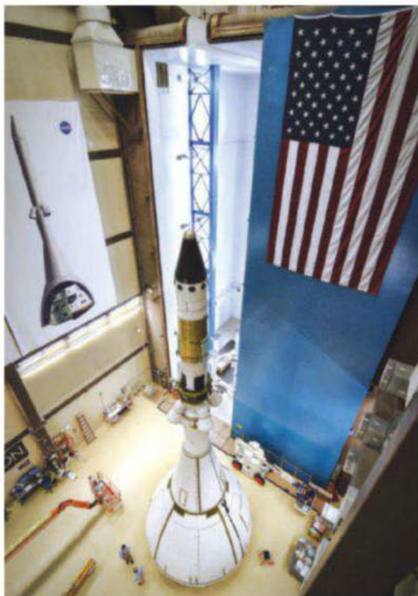
The first Orion crew vehicle, with launch abort system attached, underwent acoustic testing last summer.
