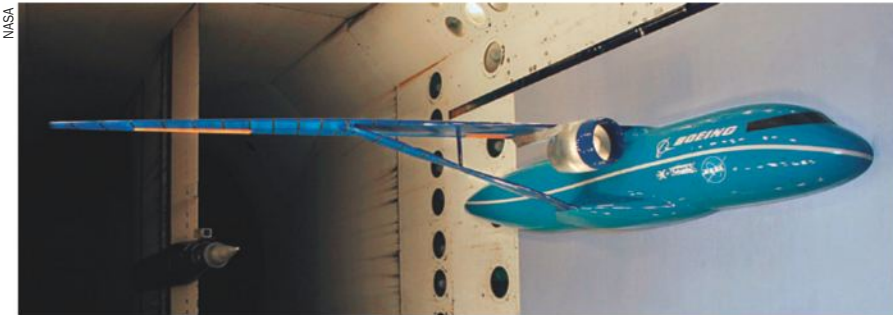
Built by NextGen Aeronautics, Boeing's Sugar High truss-braced wing model has a 12.75-ft. half-span.
