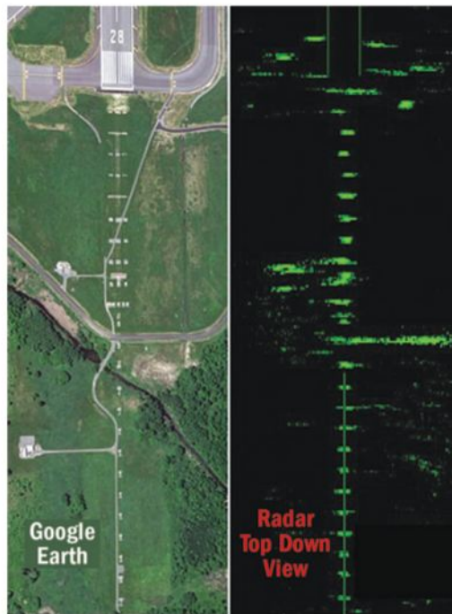
Modified MultiScan weather radar that reveals approach light structures may be part of Rockwell Collins's low-visibility landing aids in the future.
