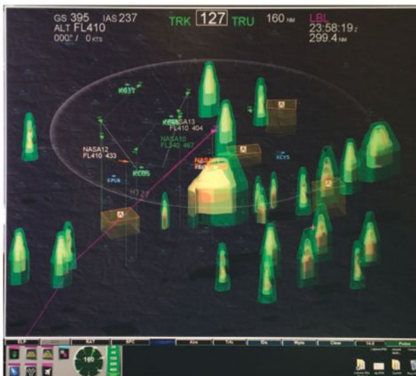
The NASA-developed Cockpit Situation Display provides a 3-D graphic of current and future weather, traffic and obstacles along an aircraft's route.
