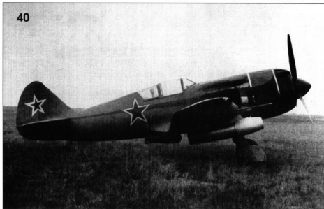
39, 40. Самолет "126ПВРД" в период проведения заводских испытаний. The Aircraft "126ПВРД" with two auxiliary ramjet engines under evaluation.
