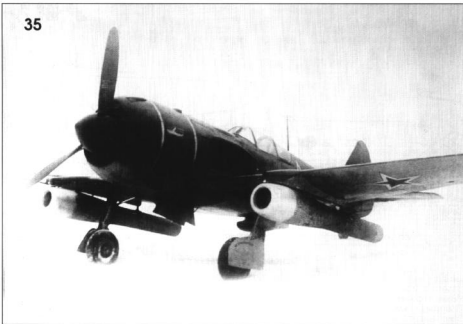
35, 36. Самолет Ла-9РД с ПуВРД Челомея. The La-9RD aircraft with two auxiliary pulse-jets.
