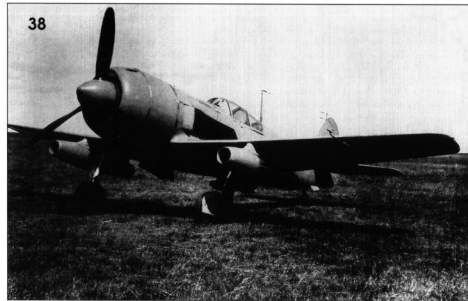
38. Самолет "138" — с ВРД-430 во время заводских испытаний. The Aircraft "138" with two auxiliary VRD-430 ramjets under evaluation.
