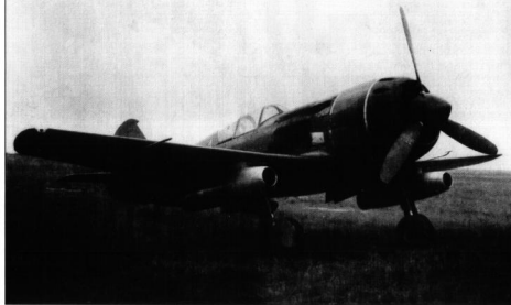
39, 40. Самолет "126ПВРД" в период проведения заводских испытаний. The Aircraft "126ПВРД" with two auxiliary ramjet engines under evaluation.
