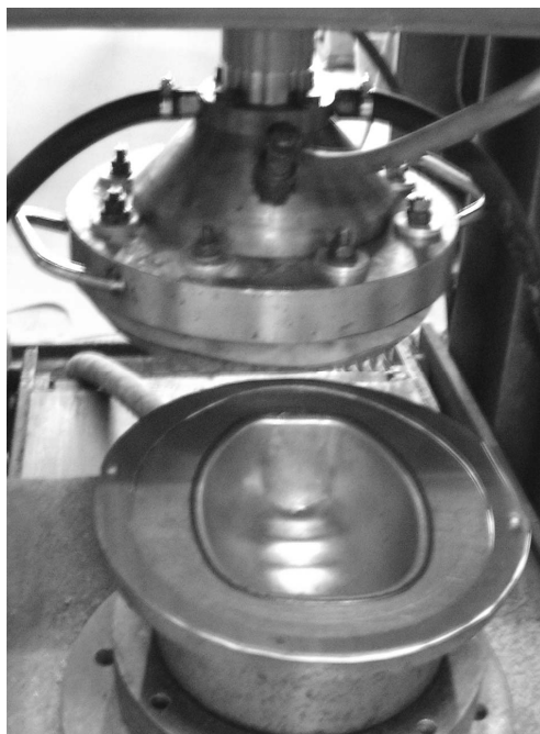
Fig. 2. Conical discharge chamber and tooling placed in technological unit of the installation UEHSh-2
