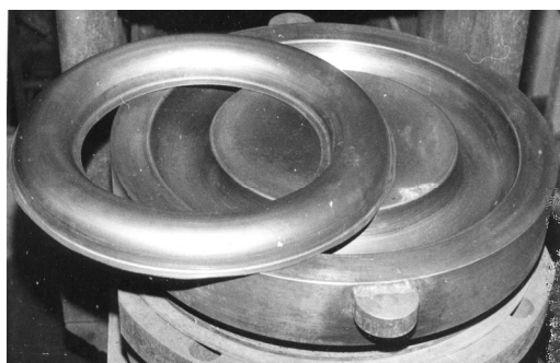
Fig. 3. General view of die and article “fairing” of 488 mm outside diameter from steel St3kp of 1,5 mm thickness
