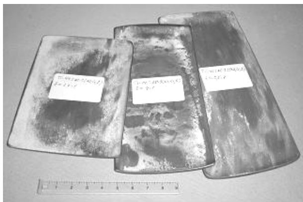
Fig. 3. Semi-finished sheet products rolled below the eutectoid temperature
