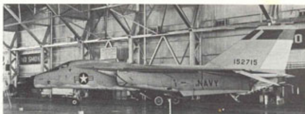
Seventh and last F-111B (BuNo. 152715) at the Navy's China Lake, California, facility in May 1971. Tail skid shows clearly in the extended position. Stripe on tail is red. Variable-sweep wing offers excellent fringe benefit of minimal parking space requirements. (Photo: Roy Lock)
