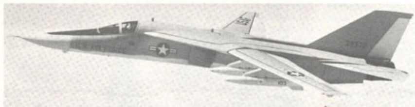
Seventh test and development F-111A (AF 63-9772) with training (dummy) weapons on undervying pylons undergoing evaluation over Texas on October 22, 1969. (Photo: GD/FW, ref. 30-31219)
