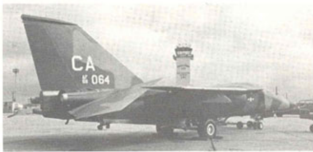
A TAC F-111E (AF 68-0064; 74th built) photographed in 1971 and wearing the old tail coding of "CA" (now "CC") of the Cannon AFB, New Mexico-based 27th TFS, 20th TFW, TAC. From the rear, the massive tail assembly including one-piece "slab" horizontal surfaces are impressive; "064" is merely visiting Bergstrom AFB, Texas. (Photo: Jay Miller)
