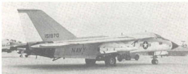
The US Navy prototype GD/Grumman F-111B (BuNo. 15970) was still going strong on May 19, 1968 at Edwards (now Flight Research Center) three years and one day after its first flight. Undervying ordnance comprises experimental- prefixed Hughes XAIM-54A Phoenix missiles. (Photo: Duane Kasulka)
