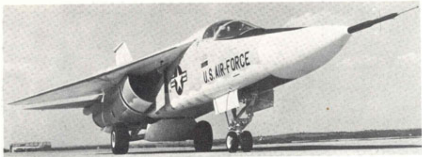
Low-angle portrait of an early GD/FW F-111A reveals the variable-geometry intake "spike" or quarter-circle centrebody which controls air flow to face of the jet engine compressor as a function of Mach No. Translating cowl is also partially open. (Photo: GD/FW, ref. 30-27337)
