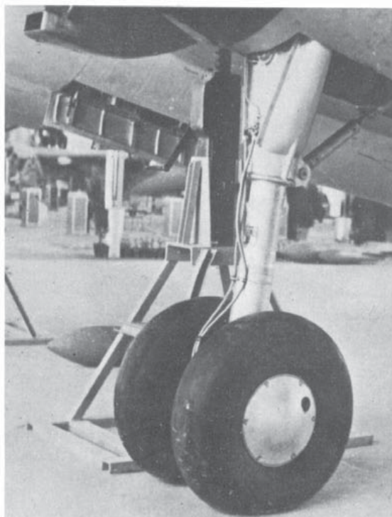
1 A close-up view of the revolutionary Kubicki main undercarriage leg of the P.37 bomber. (Photo: A. Morgała)
