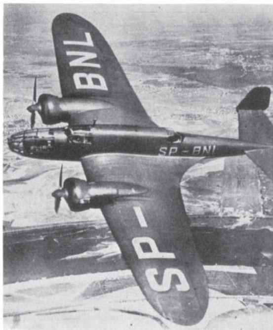
The SP-BNL over the river Vistula near Warsaw, showing to advantage its low-aspect-ratio wings, which bestowed on the bomber exceptional load-carrying capabilities.
