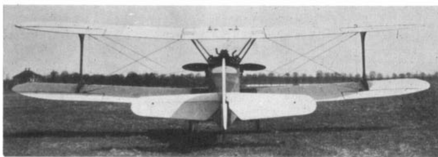
Udet U-12 prototype at Munich-Schleissheim, April 1925. The original small-area rudder and short-nose fuselage are apparent. (Photos: Udet Flugzeugbau GmbH, via Peter M. Bowers and Author's archives)
