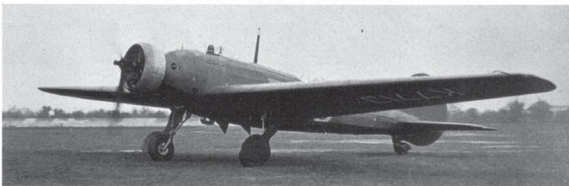
K7713 was the first production Type 287 Wellesley to Air Ministry Specification 22/35 (which superseded specification C.4/31), and was delivered to A&AEE for evaluation trials on March 4, 1937. As yet, the smooth cowling is unpainted. "Mutt" Summers is at the controls. (Photo: Vickers, ref 4947B)
