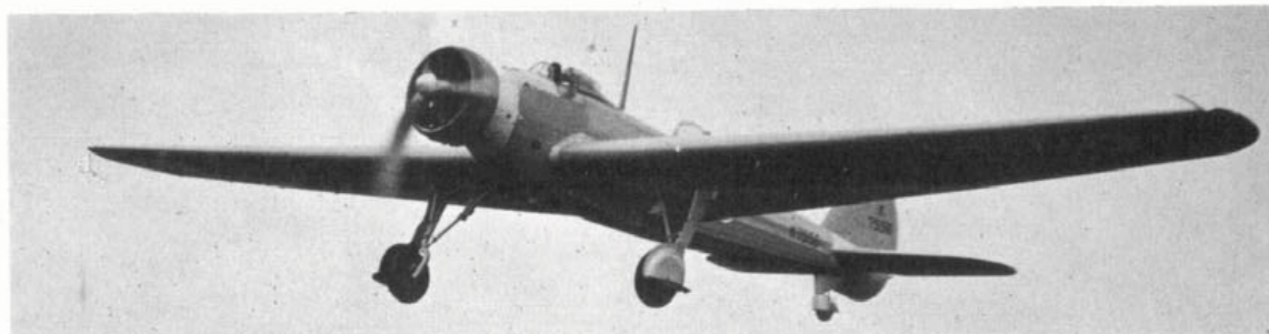
Following the Brooklands' undercarriage incident illustrated above, the PVO-9 was repaired and modified to become the Type 281 or pre-production Wellesley; now having exchanged the Class B registration for the RAF serial K7556. The fixed-pitch three-blade metal propeller fitted at this time was a Fairey-Reed unit now more readily associated with the Fairey Swordfish. Noteworthy are the upward-hinged main undercarriage leg covers; as in the cases of the Hurricane and Spitfire prototypes, this hinged section was soon discarded. (Photo: Vickers, ref. 4890-A)
