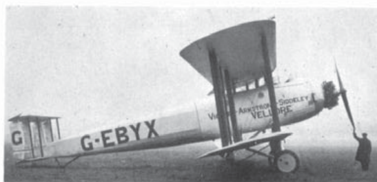
G-EBYX was a 2-seat freight and mail-carrying prototype, the Vickers Vellore, of 1928 which suggests the origins of the fuselage shape of the later, monoplane G.4/31 and Wellesley. (Below) The newly (1932) completed Vickers M.1/30 torpedo-bomber at Brooklands before application of military markings and RAF serial S1641. (Photos: Vickers (Aviation) Ltd.)
