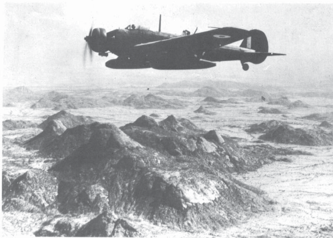
Typical of the inhospitable terrain encountered during the 1940–41 E. African campaign against the Italians. This is the only known air-to-air photograph to show the Vokes air filter under the motor cowling. The pilot's contemporary 'bone-dome' is the traditional sola topi (topee). In front of the windshield is the equally traditional bead of the ring-and-bead gunsight. (Photo: British Official via 'Flight International')
