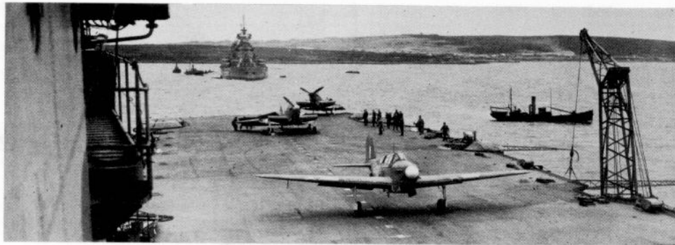
Given the brisk wind usually to be found in Scapa Flow, Fulmars could be blown off with the ship at anchor. '6-F' has its tail up after only 125 feet, with another 370 feet of Victorious' light deck ahead. The port side crane is in use for storing ship. The battleship astern is Prince of Wales. (Photo: IWM, ref. A6120)
