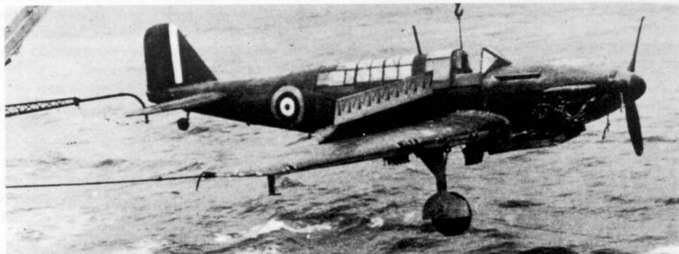
Every picture tells a story: An 808 Squadron Fulmar is suspended over the side by Ark Royal's crane, steadied by lines attached to wing tip and port wheel. The aircraft has been engaged by the barrier—hence the considerable damage to the underside of the engine cowl and radiator—and has been hoisted outboard to clear the landing area for other aircraft. Note that the flaps have not been closed before the trailing edge has been raised for folding. (Photo: via C. F. Shores)
