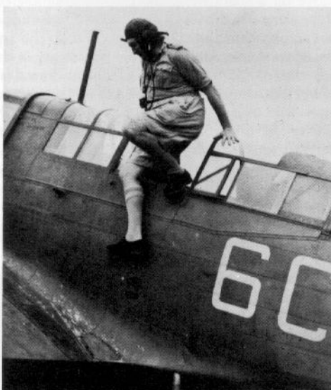
Captain T. Troubridge, RN, commanding Indomitable , climbs out of an 800 Squadron Fulmar II at RAF Port Reitz, Mombasa, after flying ashore from the carrier in June 1942. Note the sliding panels and the braced, hinged panels which gave the Observer an undistorted range of direct vision through which to take compass bearings.
