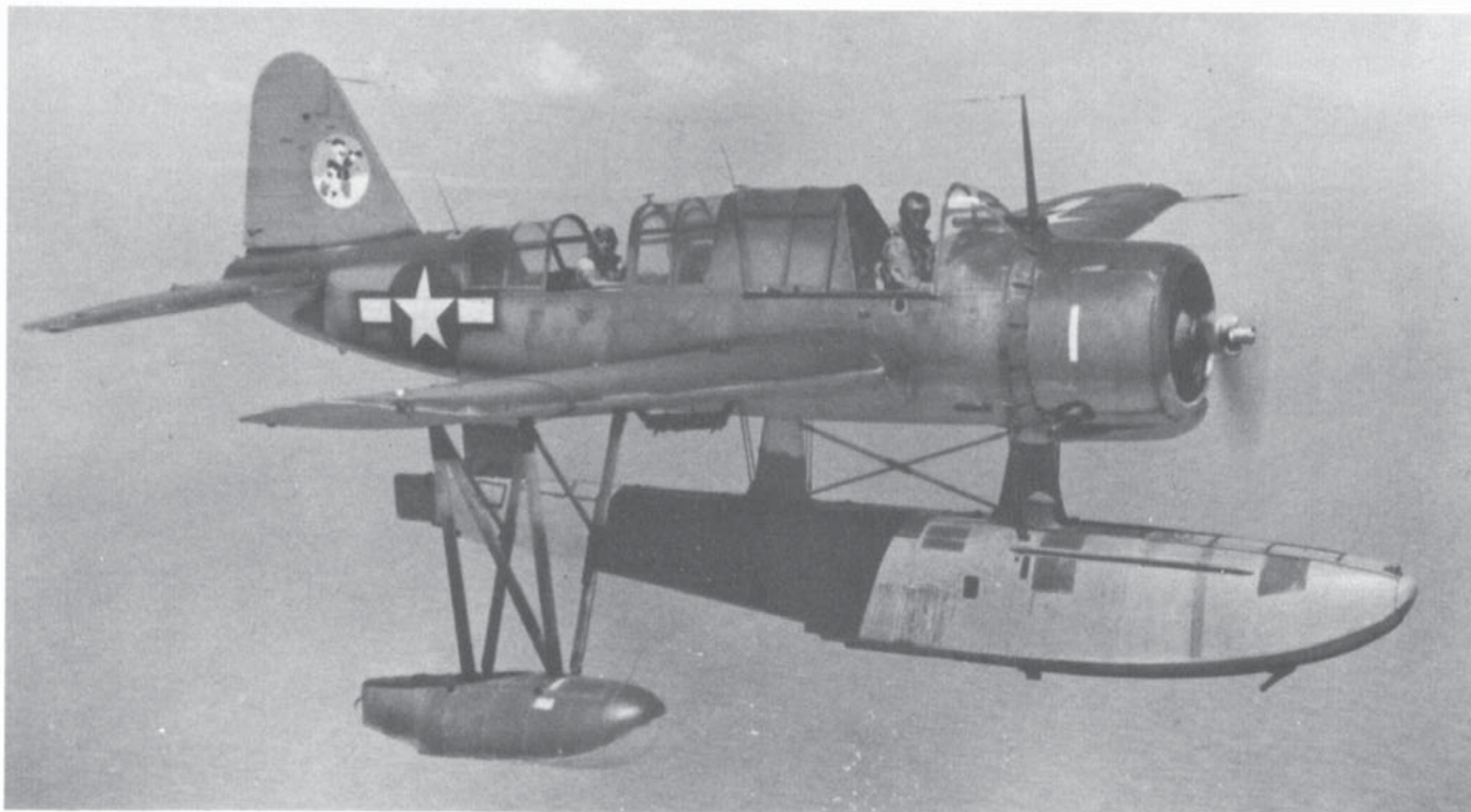
Two excellent views of unit-unidentified OS2U-3s. Fin emblem (above) shows "Donald Duck" in sailor's rig and holding a telescope. From paint weathering both OS2Us appear to have been long-service Kingfishers. The spinner (lower view) is non-standard.
