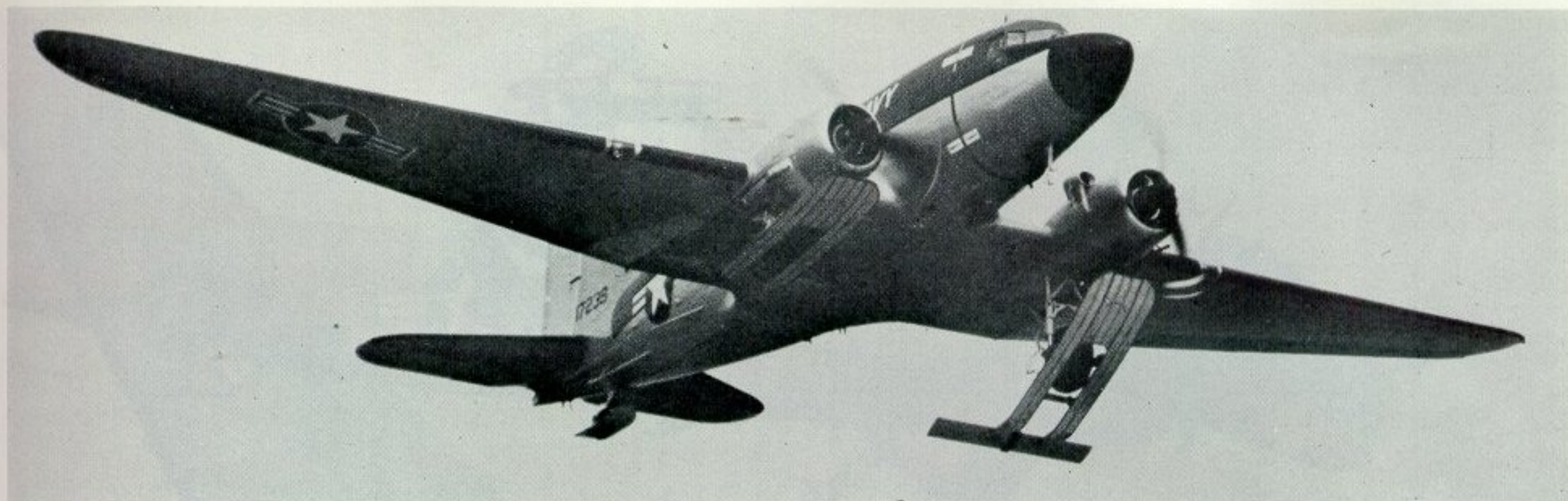
Whilst on acceptance test flight at Dallas, Texas, this R4D-5 (BuNo. 17239) developed ski trouble. It landed safely, and was later delivered to Operation Deep Freeze and VX-6 Squadron. Temco Aircraft at Dallas modified the aircraft, installed the skis, extra fuel tanks and heater units. (Photo: Arthur L. Schoeni)
