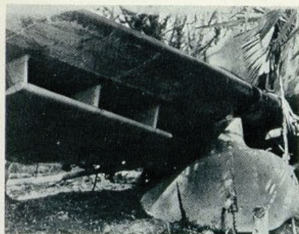
A close-up of the fixed undercarriage and dive-brake of the D3A1 carrier bomber.
