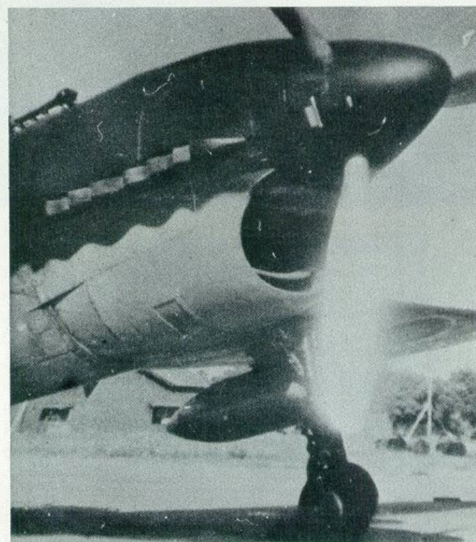
A D4Y2 in close-up shows to advantage the pilot's external gun sight and one of the two 330-litre under-wing drop tanks. (Photo: via Major Robert C. Mikesh)
