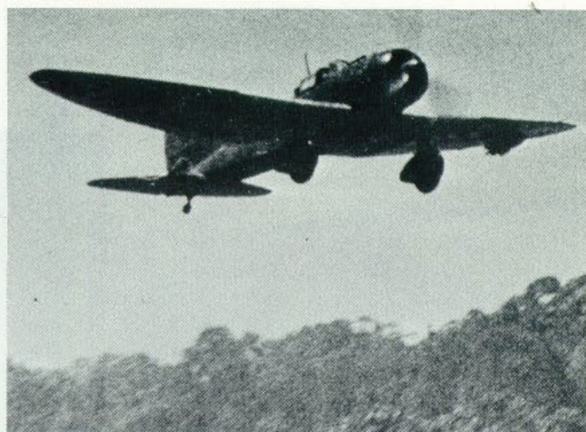
A D3A2 taking-off from one of the four airfields at Rabaul in 1943. Bomb carried under port wing is noticeable.
