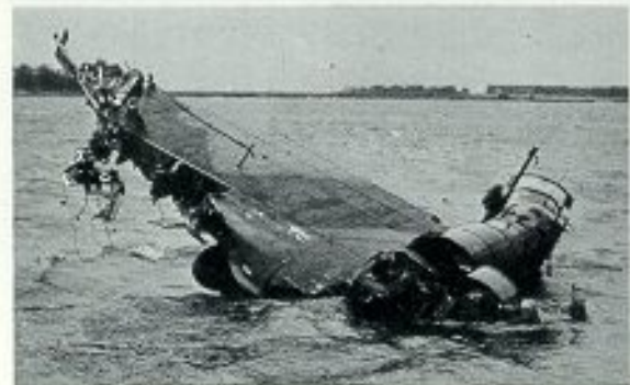
An engine fire shortly after take-off caused the loss of this Naval Air/Sea Warfare Development Unit Barracuda III, seen in shallow water less than a quarter of a mile from the end of the runway at RAF Thorney Island. Both the pilot, Lieutenant G. W. Halliday, DSC, RNVR, and the Observer, Lieutenant G. Wallace, RNVR, escaped, virtually uninjured. (Photo: G. Wallace)
