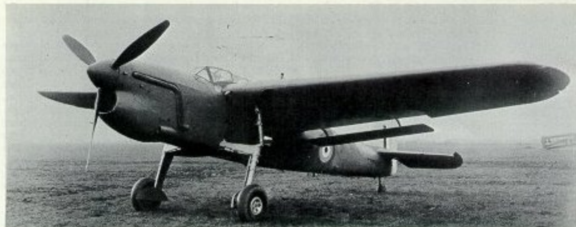
P1767, the prototype of the Fairey Barracuda in its initial clean form, as it was "rolled out" from the Hayes factory in December 1940. (Photo: Imperial War Museum, ref. 104398)
