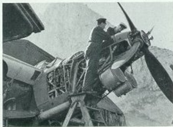
A Barracuda II of the front-line Reserve Aircraft Pool held at Gibraltar for carriers operating in the Mediterranean. The "drums" below the cantilevered Merlin 32 are the engine radiators and the oil cooling radiator (below). Surprisingly, the engine, with accessories and propeller, was nearly as heavy as the remainder of the fuselage structure.
