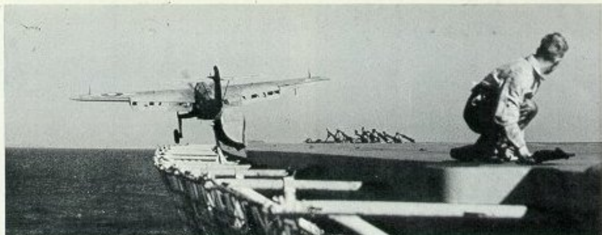
A member of HMS Vengeance's catapult crew watches the bomb-laden "378" of 812 Squadron as it leaves the catapult trolley during flying exercises off Australia in December 1945. (Photo: C. H. Wood)
