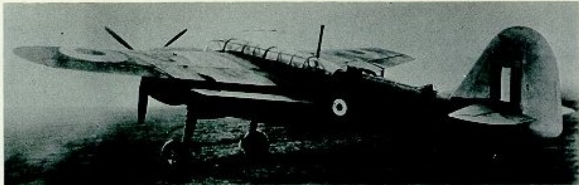
Another view of P1767, showing the Albacore-type tail unit and the original form of the flap hinges, with the jack and the two fairings above the wing trailing edge. The installation on the rear-fuselage top-decking is a spin recovery parachute.
