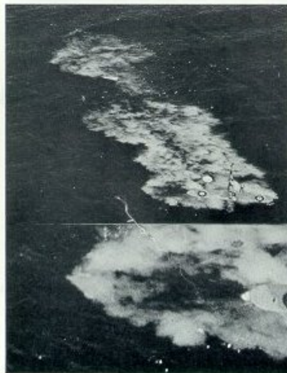
Nobody has got their feet wet, yet! The crew of an 812 Squadron Barracuda—the pilot on the trailing-edge of the port wing, Observer leaving his cockpit, and TAG preparing to haul the circular dinghy in. The sequence of the ditching can be seen in the inset, the furthest disturbance marking the first bounce as the aircraft touched the water, tearing off the starboard flap. (Photos: C. H. Wood and G. Wallace)
