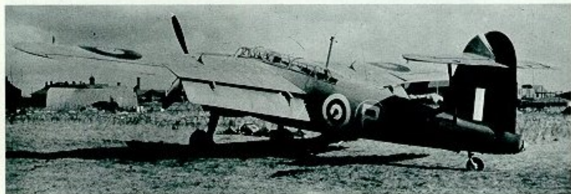
P9642, the first production Barracuda I, seen in April 1942, on the hard-standing of what is now London Airport (Heathrow). Patches cover the position of the wing locking pins, removed in order to assess the difference in performance; as this amounted to less than two knots, the decision was made to retain the fixed installation, rather than replace it with retractable fittings.
