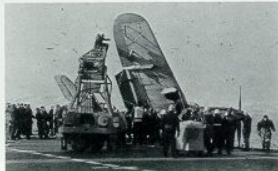
"Jumbo", the mobile crane, is conned towards one of 812's aircraft which has come to rest in Vengeance's port deck-edge catwalk after the port main undercarriage leg had collapsed during a landing. (Photo: C. H. Wood)
