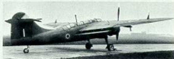
P9976, the initial Griffon-Barracuda, a Mark II from the first production batch modified to accommodate a Rolls-Royce Griffon VIII engine, and with an extended dorsal fillet to compensate for the opposite (to the Merlin) propeller rotation and the extra length of the engine cowling.
