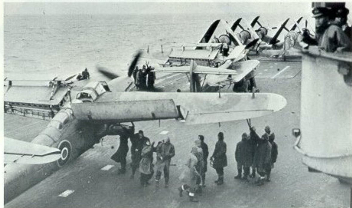
"4A" (LS350, the flagship of No. 52 TBR Wing (829 and 831 Squadrons), folds its starboard flap and inboard trailing edge preparatory to the wings being folded. Note that the TAG's lower window has been removed and replaced by a "solid" panel. (Photo: Imperial War Museum, ref. Q23038)
