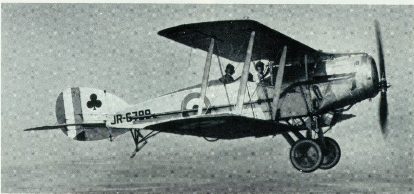
Rebuilt F.2B, JR6788 of 208 Squadron, flying over Suez Canal area. This particular aircraft has been locally modified by removing the gunner's Scarff ring and fairing over the rear fuselage, possibly for use as a unit "hack" communication vehicle. The Flight markings of a black "Club" on a white circle (denoting A Flt.) was doped on fin, upper centre section and under starboard lower wing.
