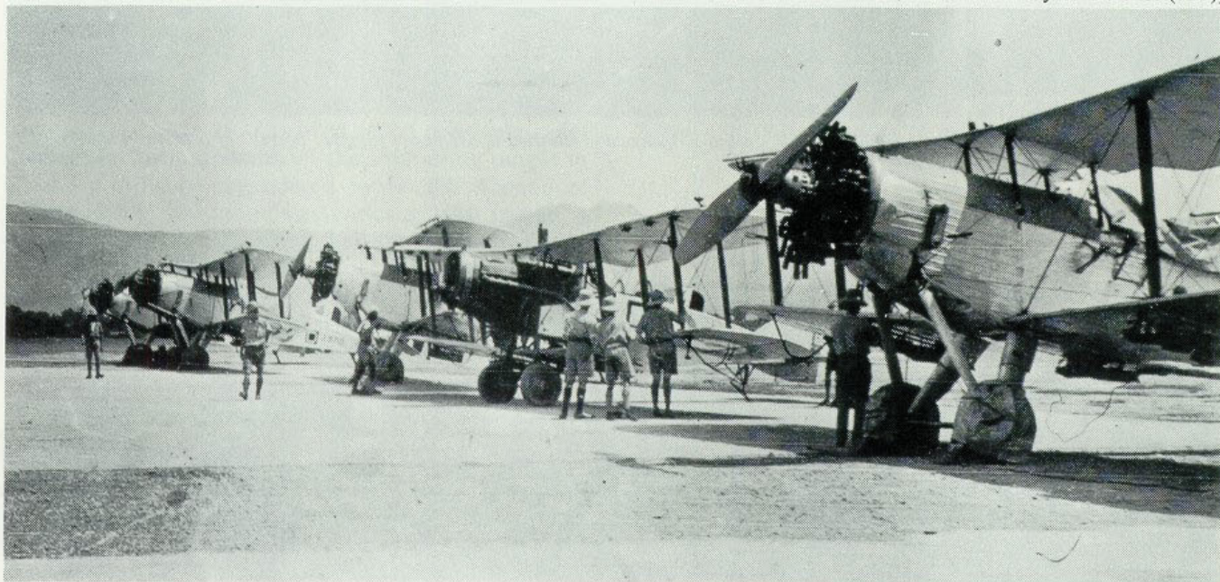
"A" of 28 Squadron preparing for take-off at Secunderabad India, on January 17, 1931. Of particular interest are the "desert" tyres, tropical radiator and upper wing centre-section cooling outlet piping. (Photo: courtesy No. 28 Squadron, RAF)
