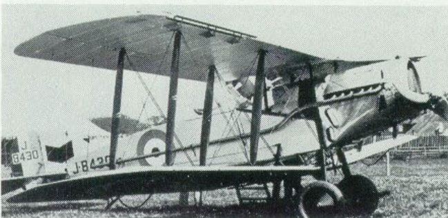
J8430 was the second F.2B built of a batch, J8429—J8458, specially converted to two-seat, dual control and completed between January and June 1927. This particular F.2B was further modified to include large rear cockpit windscreen and upper-wing auto-slats. Wheel covers were doped in red; while aircraft was brought onto the strength of No. 24 Squadron for maintenance purposes, as a personal transport for the use of Edward, H.R.H. The Prince of Wales, later H.M. King Edward VIII.
