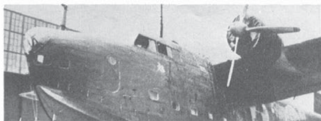
A H8K2-L Seiku (Clear Sky) Transport Flying-Boat which has retained the nose turret of the H8K1 series. (Photo: I.J.N.)
