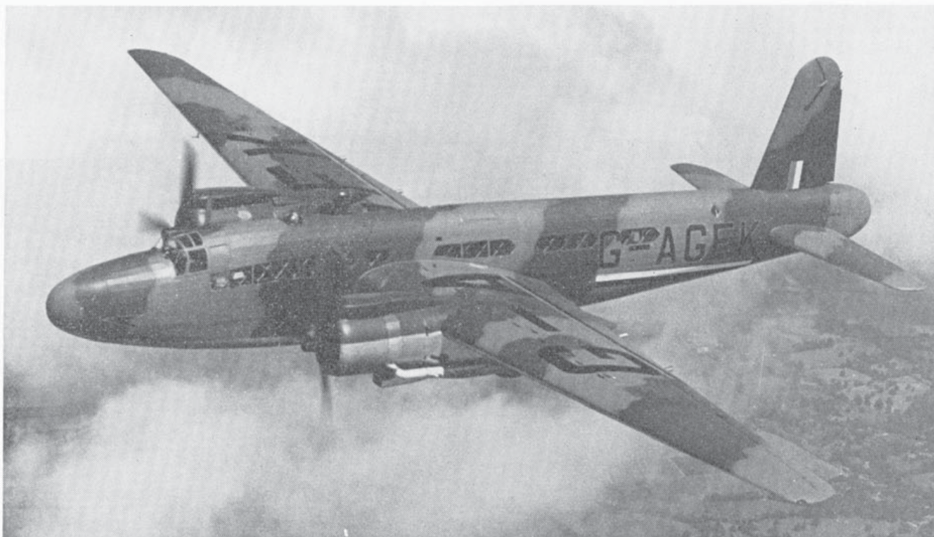
G-AGFK, the last of 14 Warwick C.Mk. Is converted for BOAC. This aircraft and G-AGFJ had cabin windows different from the remainder of the fleet. (Photo: Vickers)
