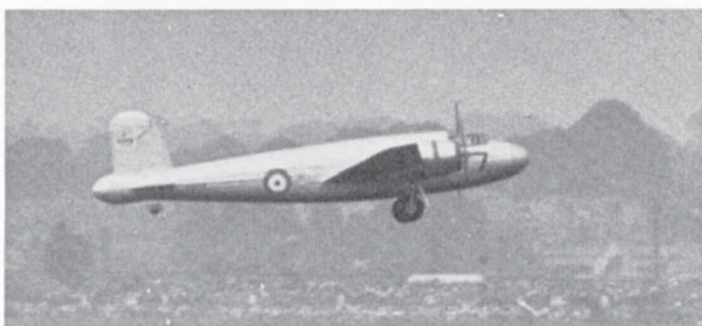
K4049, the B.9/32 prototype of 1936 that preceded the production Wellington bomber which was an almost total re-design—benefiting substantially from the contemporary Warwick.
