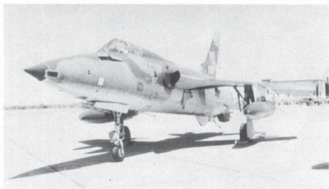
The sixth Thunderchief of this block, F-105B-20RE (57-5808) was photographed at McClellan AFB, California in May 1969 and bears the badge and unit markings of the 561TFS/23TFW. Unlike the later F-105D/F variants, the F-105B has a shorter radar nose cone and forward-positioned cannon port for the 20-mm M-61 Vulcan. Also clearly visible is the partially opened cover to the flight refuelling probe. (Photo: Author)
