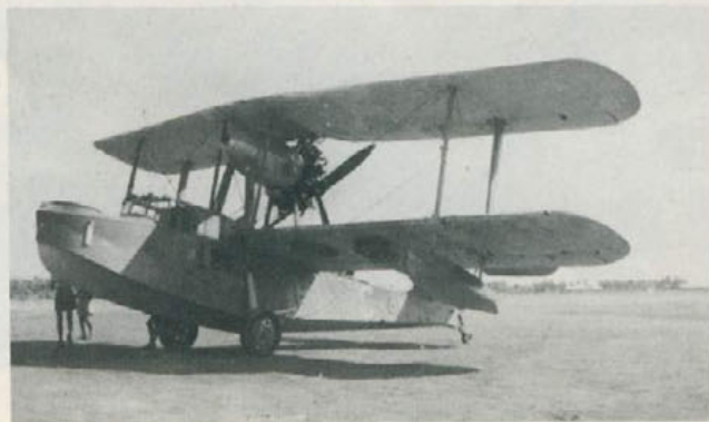
Below "C" of 700 (Mediterranean) Squadron at Fayid, in the Suez Canal Zone, prior to the fitting of ASV radar in the spring of 1942, but with the brackets on the interplane struts and the sockets in the leading edge of the upper mainplane. The full serial is indistinguishable, but the last three digits are —44G, from which it may be inferred that the aircraft has at least some of the internal ASV equipment.
