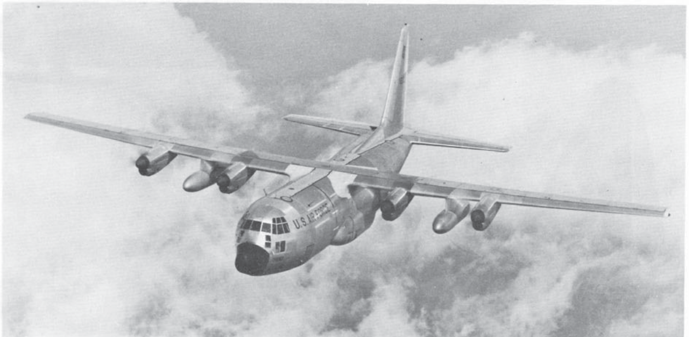
Another view of the same USAF C-130E as that shown in the previous picture, illustrating the compact installation of its 4,050 eshp T56-A-7 A turbo-props.
