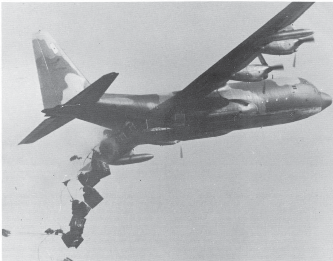
Another USAF C-130A, paradropping supplies into a Vietnam combat zone during an early stage of the war, for U.S. Army ground forces. As can be seen, the fuselage is of constant width right up to the point where it meets the tailplane. (Photo: U.S.A.F.)
