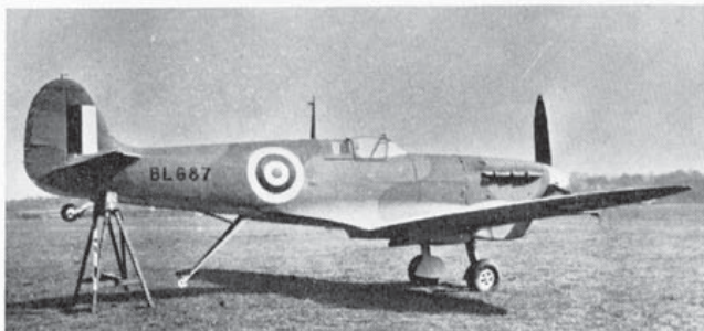
Hooked Spitfire Mk. VB BL687/MB329 resting on trestle, clearly showing the arrestor hook in lowered position. (Photo: Real Photographs, Liverpool)
