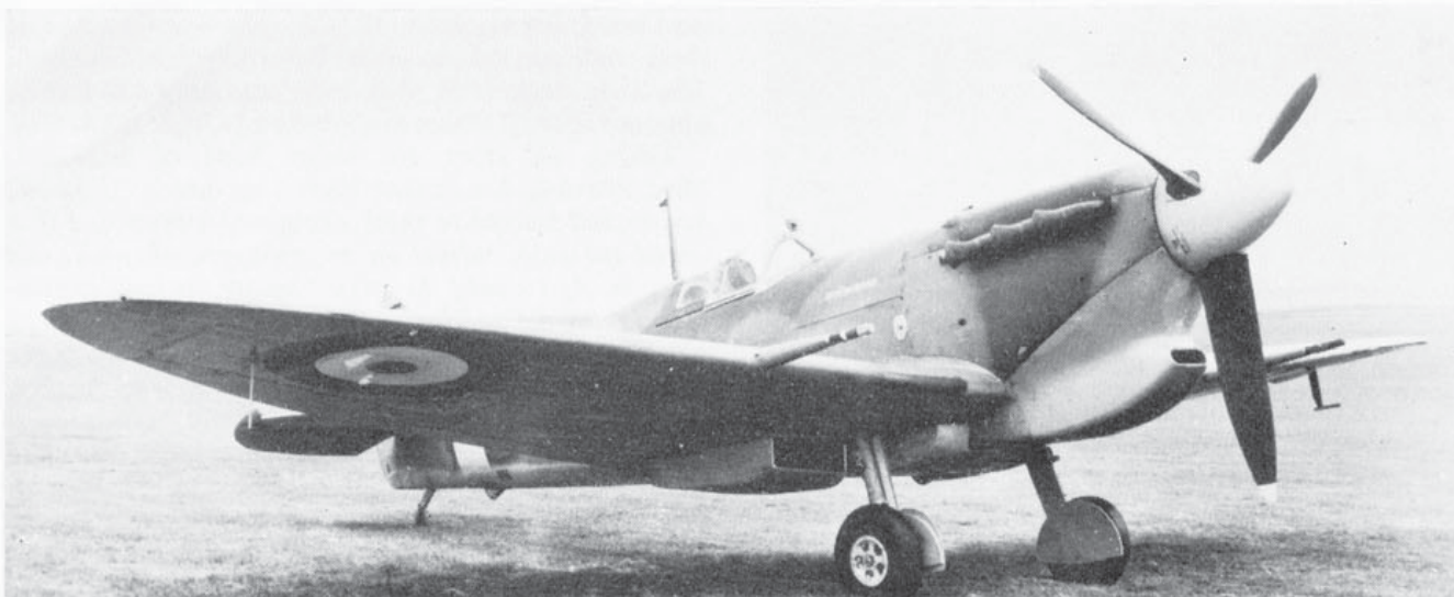
Hooked Spitfire Mk. VB named Bondowoso (military serial BL676/MB328). Note this first converted Spitfire, to Seafire Mk. IB standard, carries a 30-gallon slipper tank under the fuselage and is fitted with a tropical filter.
