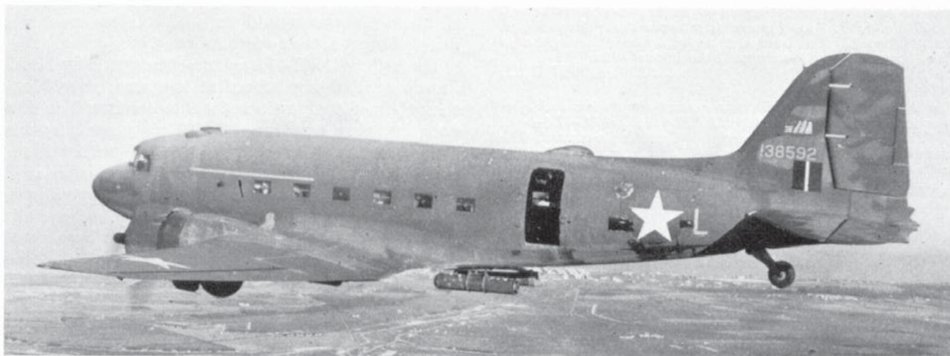
Carrying an R.A.F. fin flash this Santa Monica-built C-47-DL 41-38592 c/n. 4541 is one of the many of its type which served the Allies. Note the supply cannisters carried on external racks below the fuselage. After World War II, it served in South America before delivery to the French Air Force in 1957.
