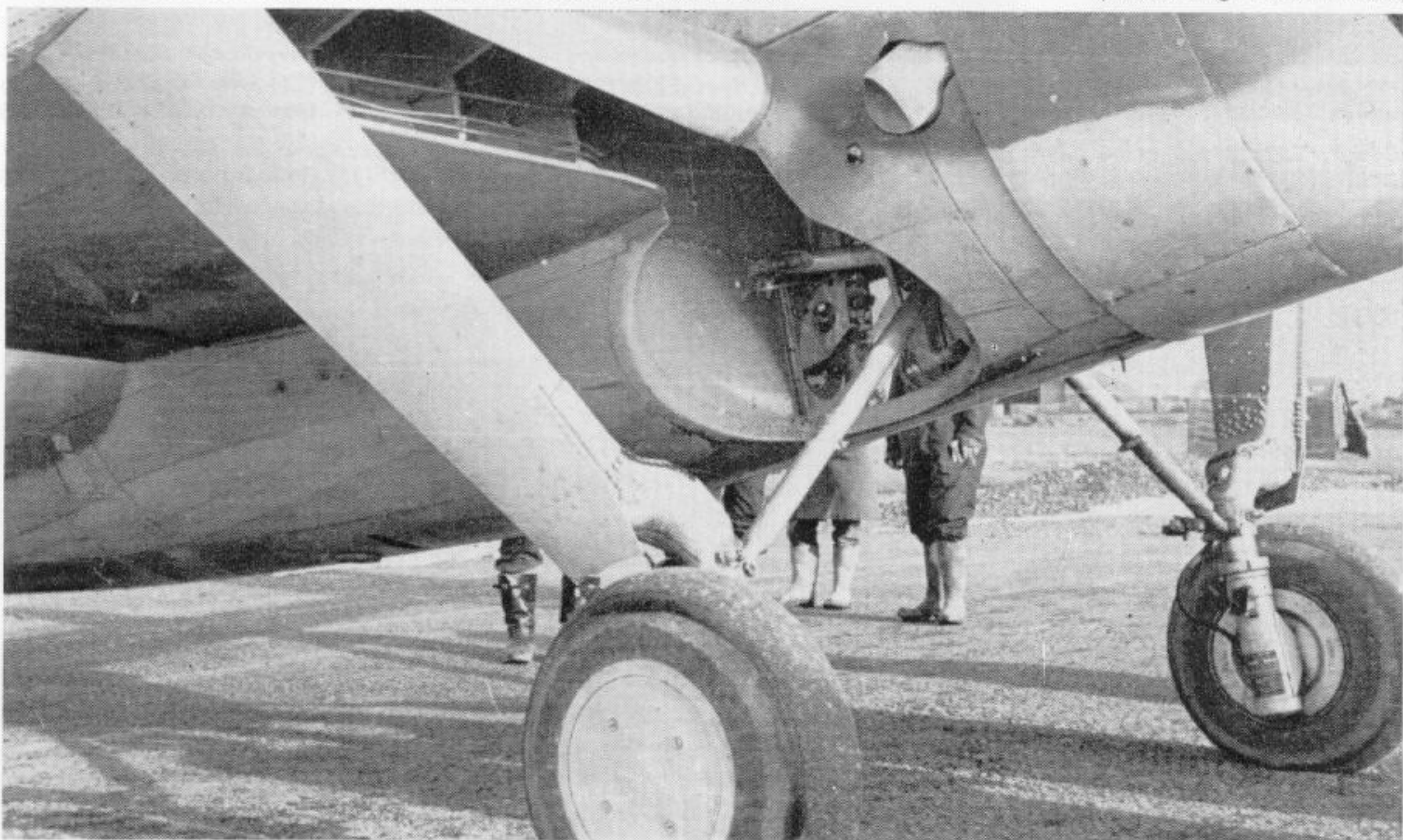
Detail of the rather unusual configuration of the undercarriage of the Buffalo.
