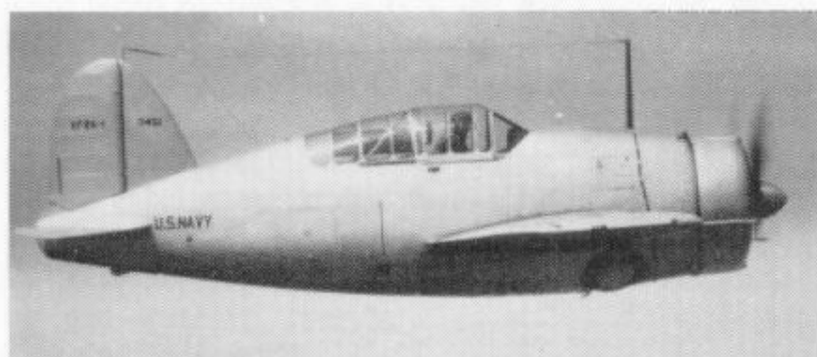
Prototype Brewster XF2A-1 in flight; note original lower-profile cockpit canopy. (via C. Macomber)
