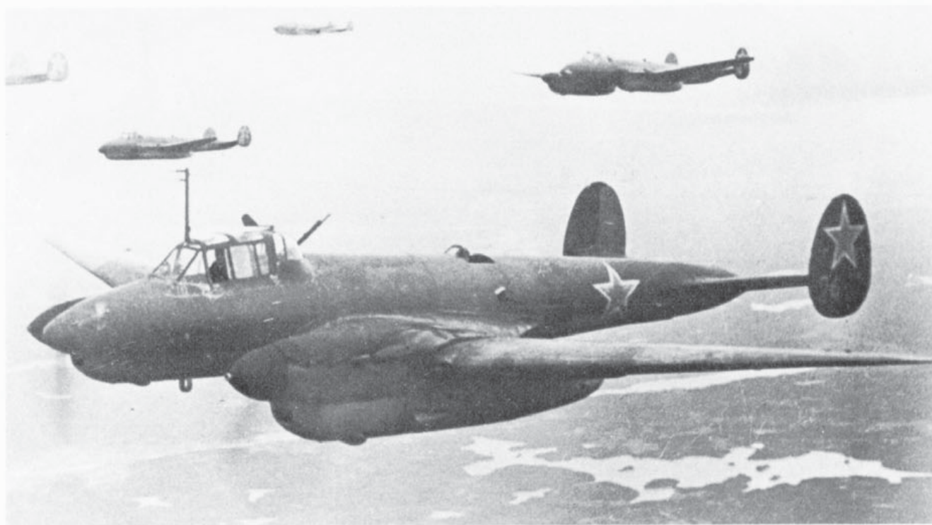
The definitive Pe-2. Period, Autumn 1944. Above the wing root can be seen the open hatch—complete with windshield—and the head of the radio operator/ventral gunner. The porthole gun just below this hatch appears to have been censored. (Photo: via Air-Britain archives)
