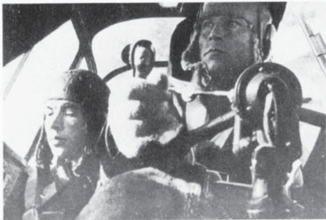
Interior 1: Photographed from inside the Pe-2's nose, the pilot's semi-spectacle control column and head protection armour are noteworthy. (Photo: via Jean Alexander)
