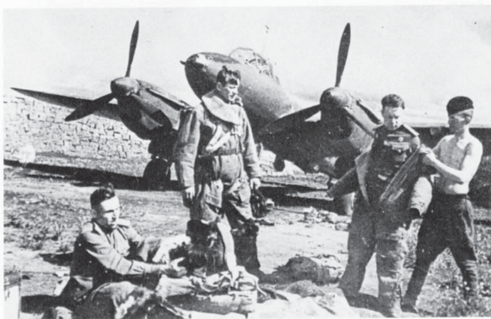
Another intermediate production Pe-2 illustrating the FT dorsal turret with rear-positioned aerial mast still retained. Once airborne, those heavy flying suits would be welcomed.
