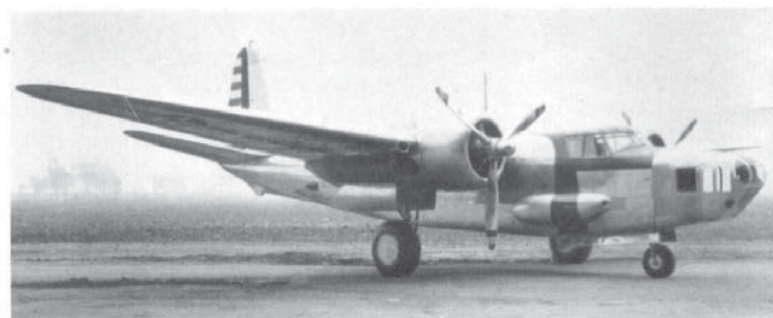
The alternative bombardier nose of the 7B is shown here.
