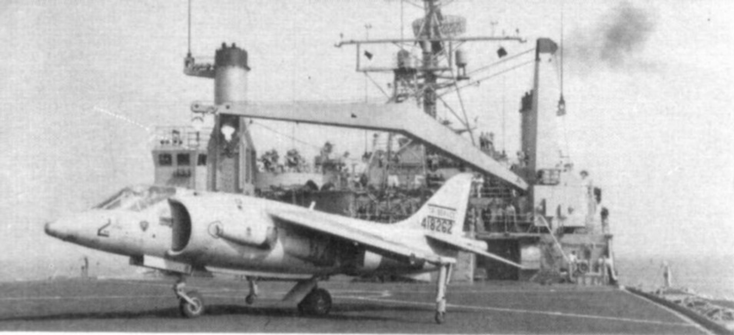
An XV-6A (Kestrel) undergoing qualification trials aboard U.S.S. Raleigh LPD-1.
