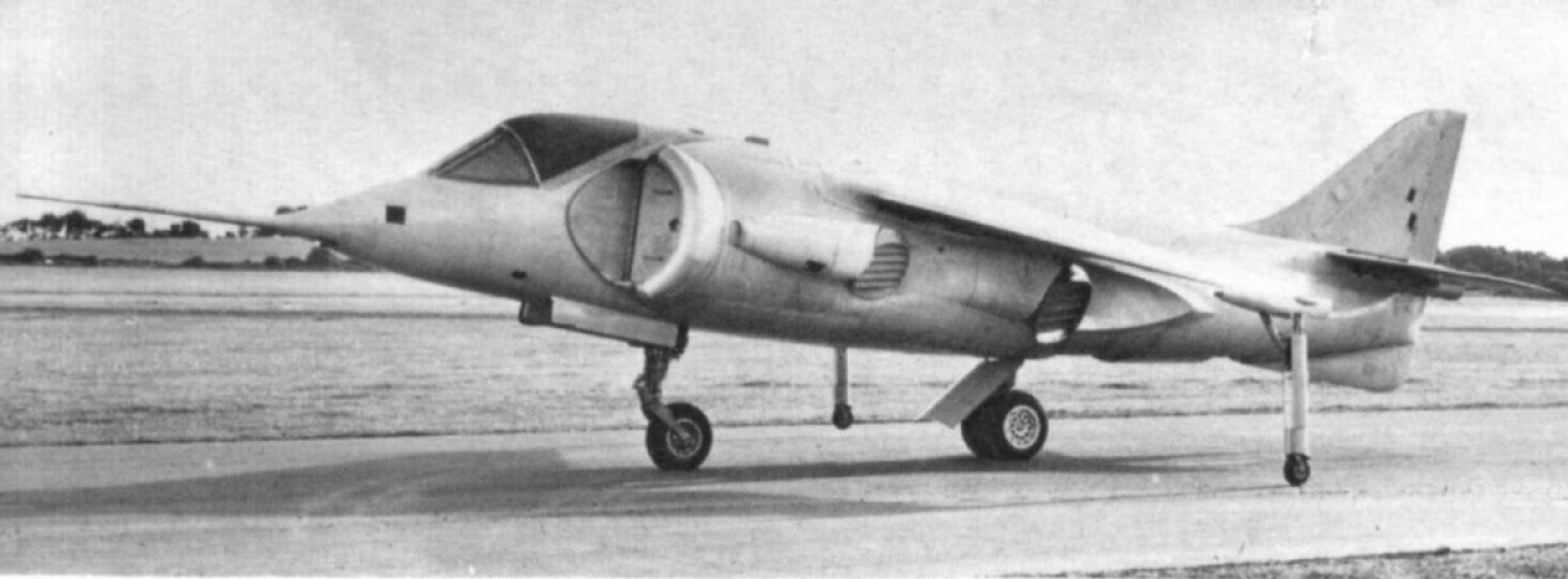
Roll-out picture of the first prototype P.1127, XP831, taken on 17th August 1960. The cockpit canopy is still protected by masking material and various minor panels are not fitted. (Neg. No. EXP255/60)
