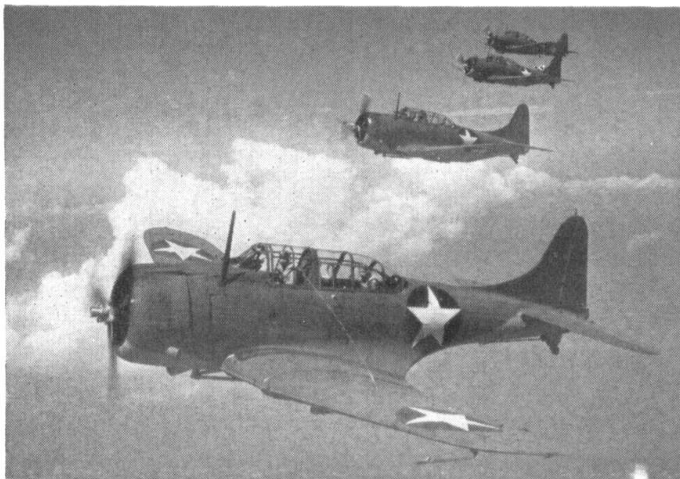
A formation of early SBD-3's; a second rear gun, improved armour and self-sealing fuel tanks carried the top weight to 6,350 lbs.
