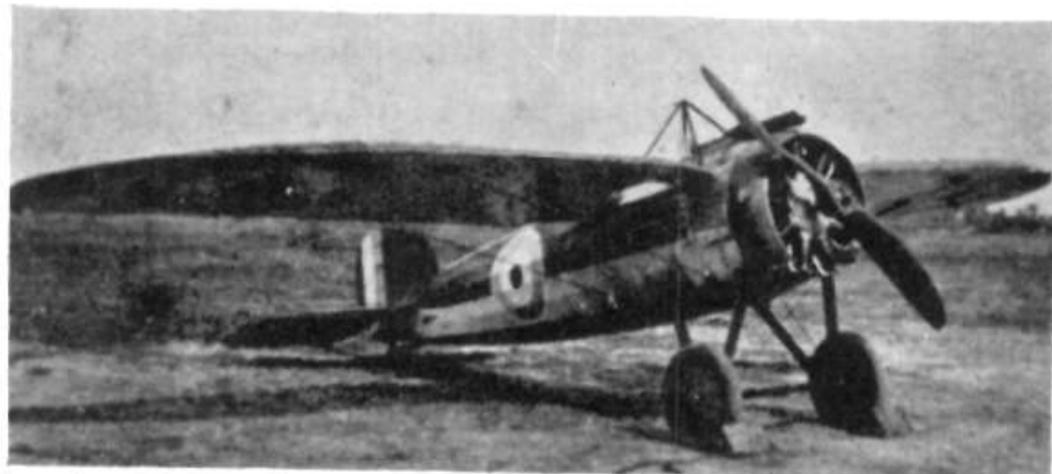
Another M.1C of No. 150 Squadron, with its spinner removed to improve cooling of the engine. This aircraft had tyres of thicker section than was standard.
