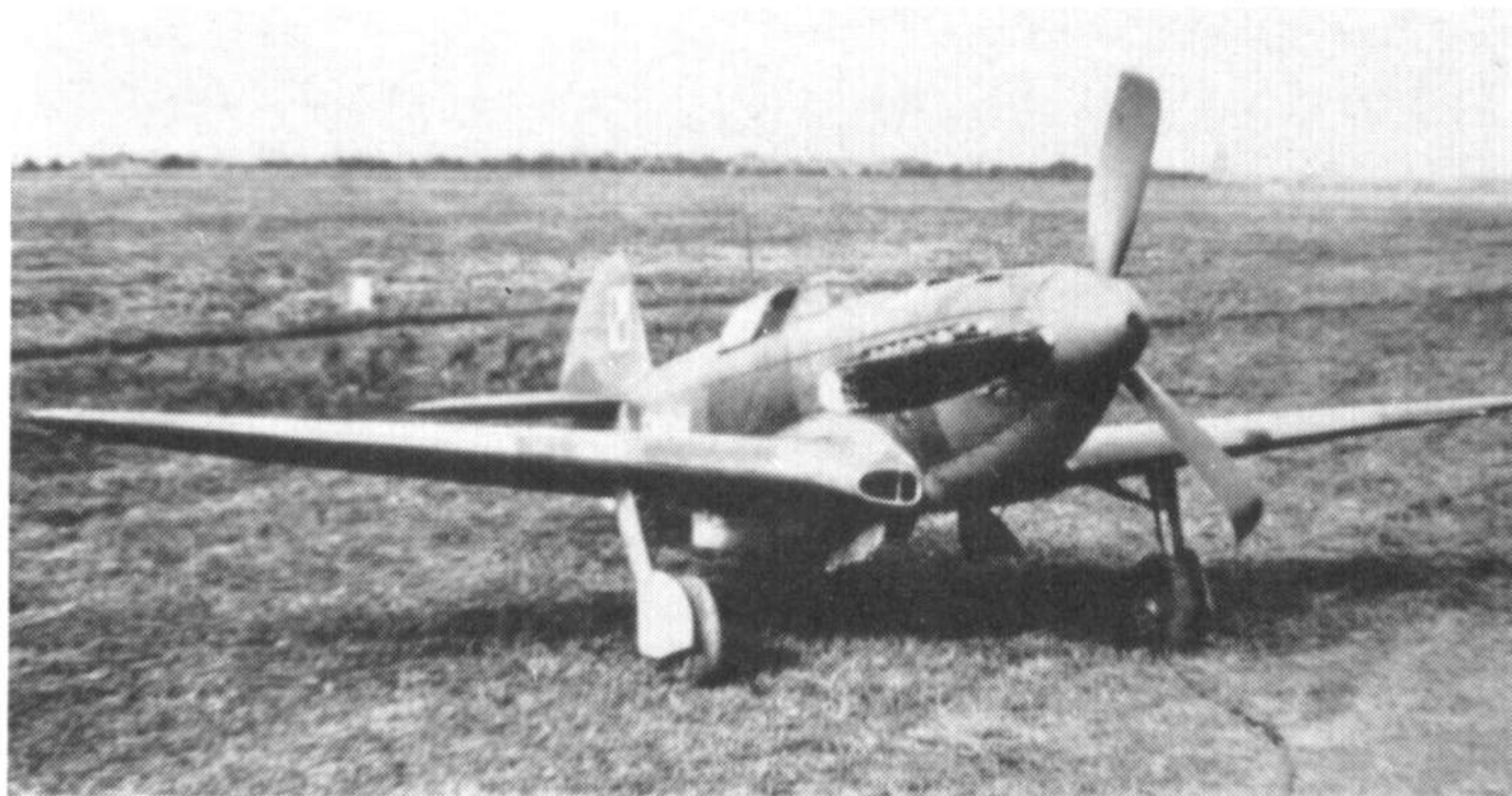
Yak-9U's in Russian (above) and Polish (below) insignia. The Polish machine was damaged in a forced landing, as evidenced by the bent propeller blades. (Photo: V. Nemecek)
