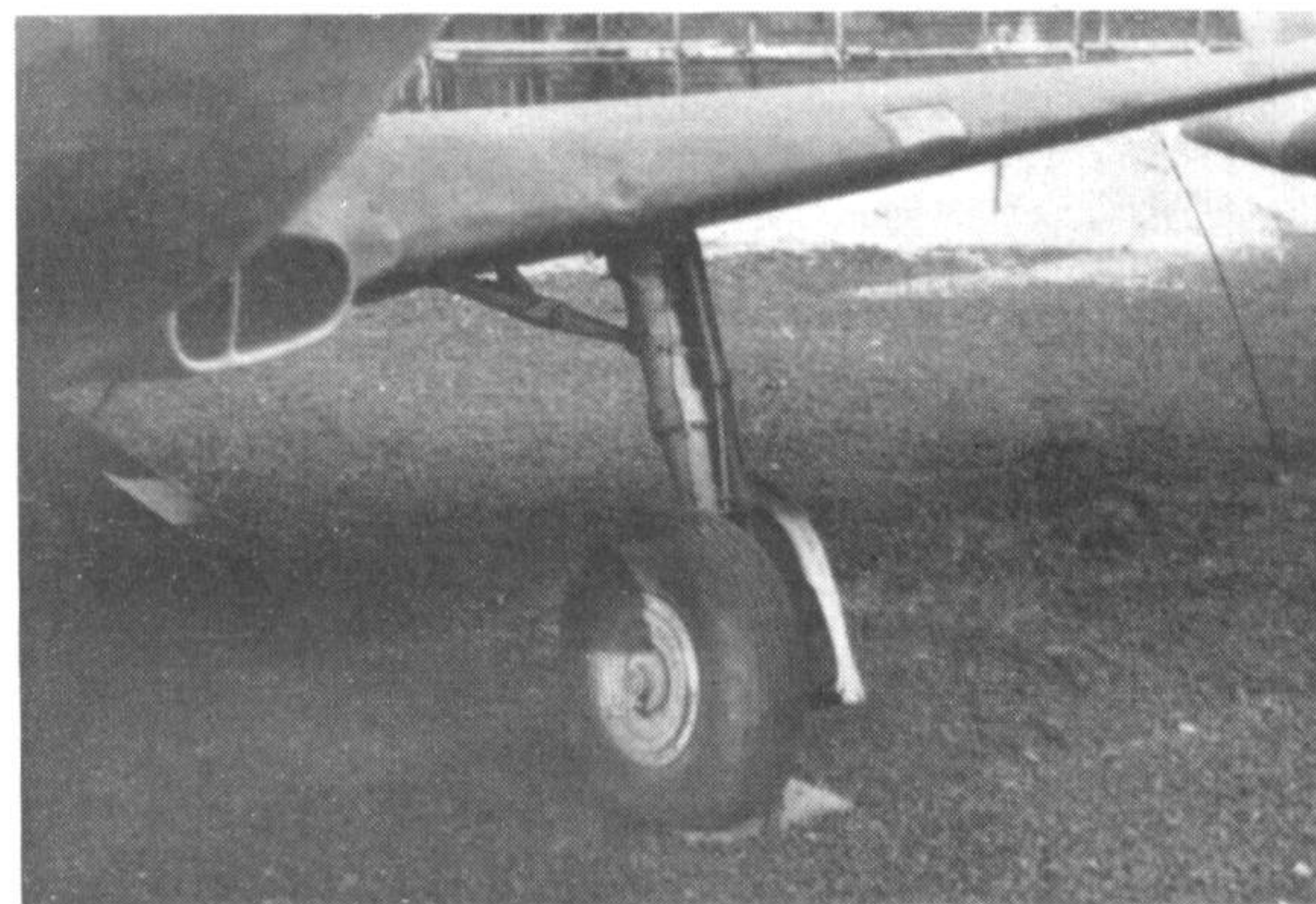
Close-ups of the Yak-9P in the Polish Armed Forces Museum, Warsaw: (top) engine cowling, showing breech and muzzle fairings of one of the machine-guns; (centre) tailplane and tailwheel; (bottom) oil cooler intake and port mainwheel leg. (Photos: the author)
