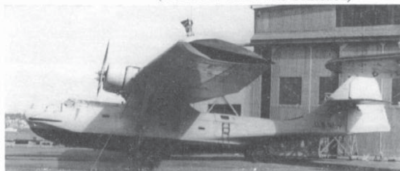
Two views of the original XP3Y-1 (BuNo 9459); in both these photographs the hull is painted light grey, not silver. (Above) The aircraft in March 1935 and (below) with additional area at the trailing edge of the rudder.
