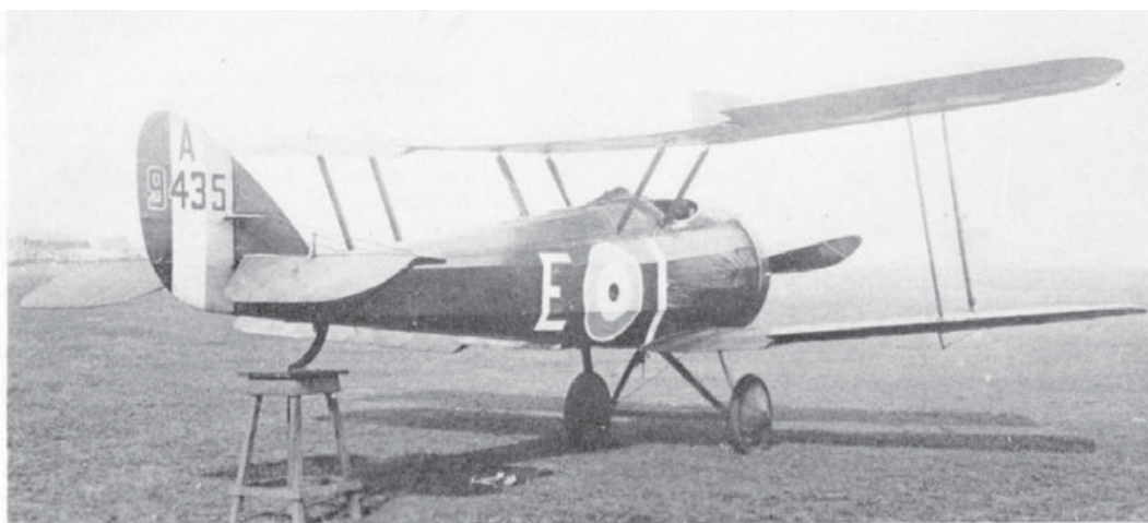
A9435 of No. 24 Squadron was captured intact by the Germans and is here seen at Adlershof. This aircraft had the stiffened engine cowling and full-span aileron balance cables in place of the earlier rubber-bungee return springs.
