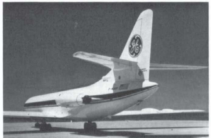
The first fan-engined Caravelle (c/n. 42) shown (above right) in original Series III form as F-WJAM , and (below) after re-registration as N420GE and re-engining with CJ805-23C's by General Electric.
