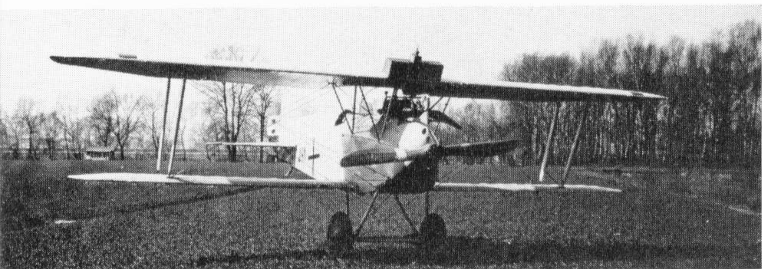
Two views of J.41, the prototype D.III (230 h.p. Hiero). Initial production of the D.III was earmarked for the Austro-Hungarian Navy and this aircraft carried late-style crosses and naval serial and markings. (Photo above: Peter M. Grosz)
