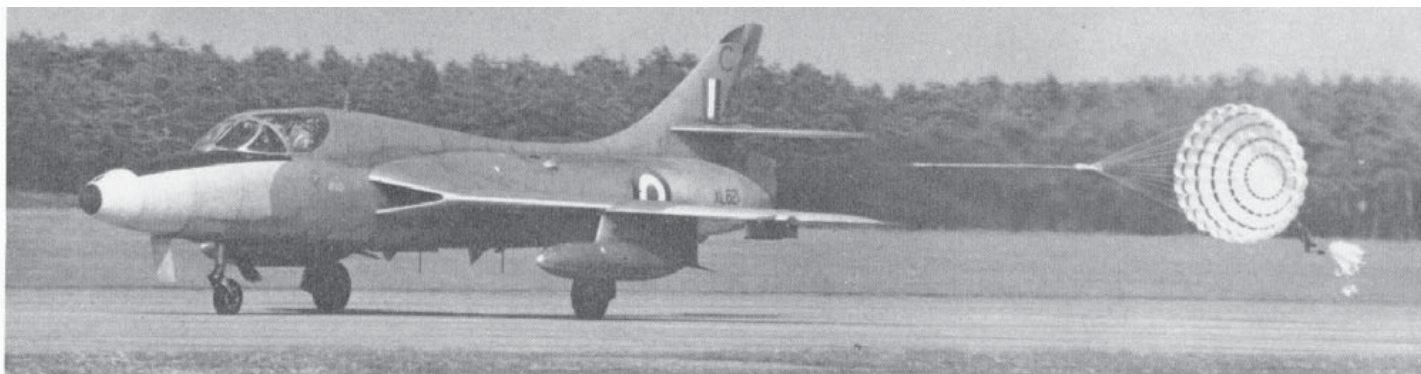
Hunter T.7 XL621 of Gutersloh Station Flight provides a fine landing study with braking parachute deployed.
