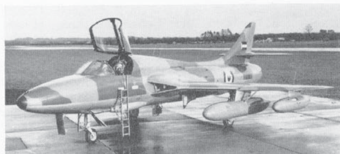
Left: Peruvian Hunter T.62, 681. Note the dorsal radio compass fairing. (Photo: Hawker, Neg. No. HTG.34/59). Right: Indian Hunter T.66, BS366. (Photo: J. M. G. Gradidge).
