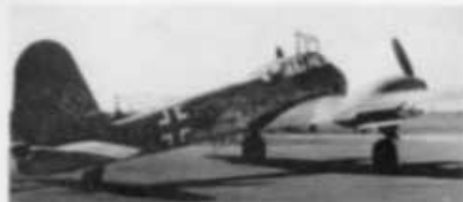
A late production Me 210A-2, W.Nr. 420098, 'PP + VO' with the FDL 131 barbettes removed. (It appears that an attempt has been made to "touch in" the barbettes on the print).
