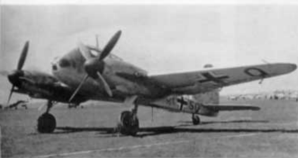
The Me 210 F11 was specially modified as a prototype for the Me 410, with four-bladed airscrews and a pressurized cockpit. (Photo: H. J. Nowarra)
