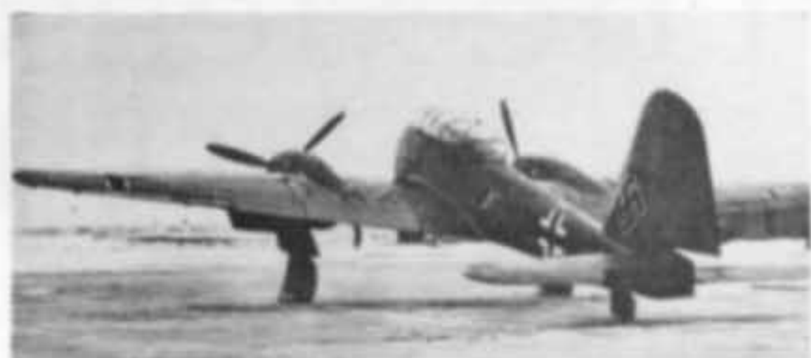
The revised cockpit and single tail of the second prototype, Me 210 V2. Despite the modified tail the machine was extremely unstable, and crashed during flutter tests on 5th September 1940. (Photo: H. J. Nowarra)
