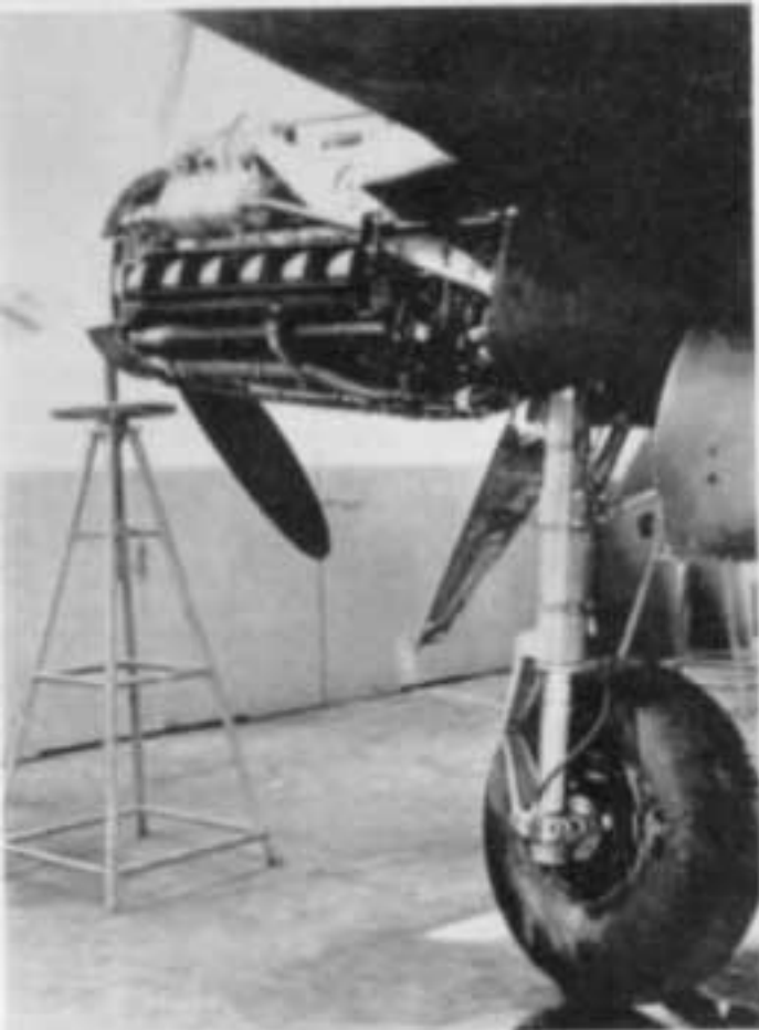
An interesting sequence showing the retraction of the Me 210's main underscarriage.
